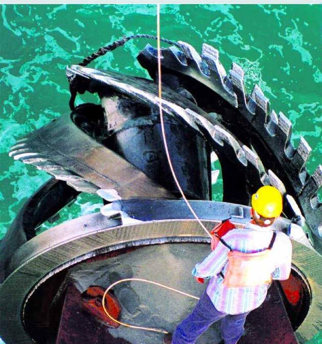
Cutter suction head for rock dredging, Qatar
